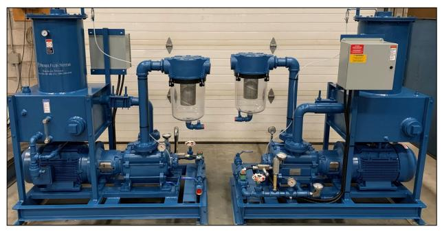
Dynaseal Vacuum System: TRVX 657/1-C/A3 with a 20 HP, 1750 RPM motor
