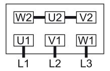
Star connection, multi-voltage motor with 9 pins (high voltage):
