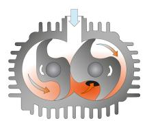
The machine works on the claw principle.
